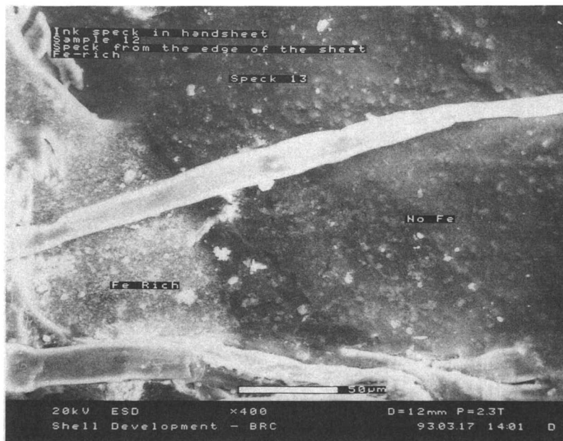
Figure 12. ESEM image of an ink particle resulting from agglomeration of an iron-containing toner ink particle and another ink particle containing no iron compounds.
