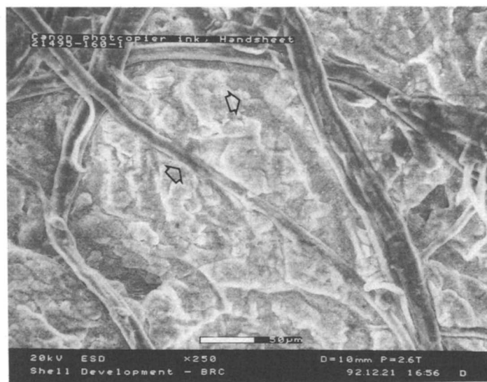
Figure 9. ESEM image of a polyester resin toner ink particle containing attached fibers after pulping in the presence of a proprietary surfactant.
