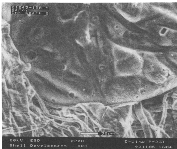
Figure 10. ESEM image of a styrene-acrylate toner ink particle after pulping photocopies in the presence of a proprietary surfactant.
