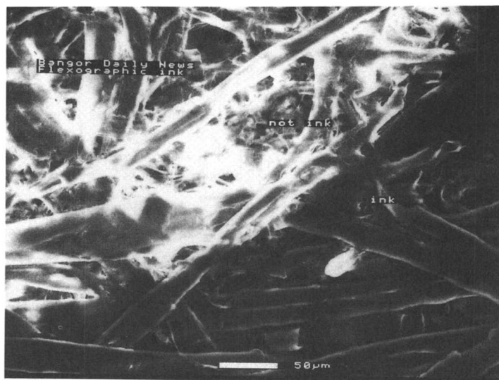
Figure 3. ESEM image of flexographic printing on newsprint.
